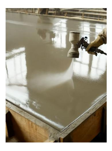
The release agent for environmentally friendly and efficient demolding.
